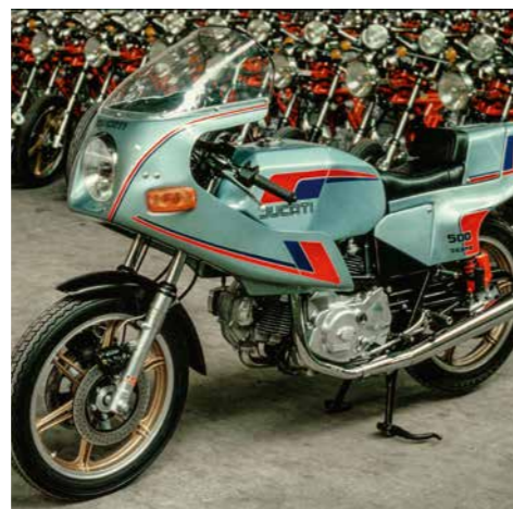
The 500 Pantah, equipped with a new belt-driven system and a trellis frame, is presented to the public.
