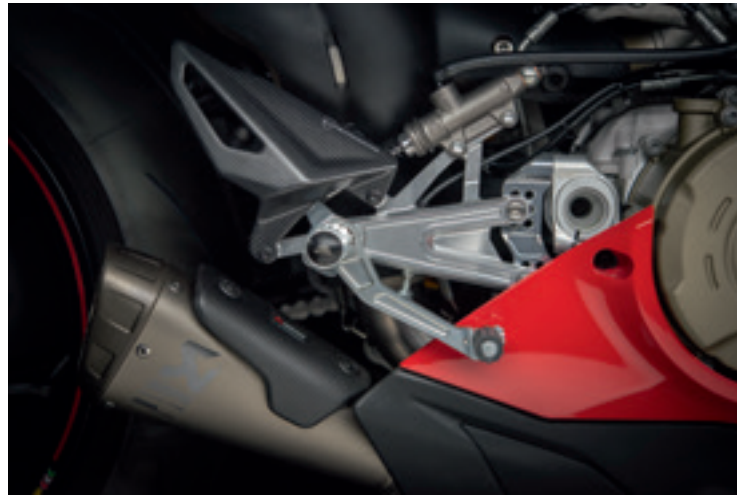
Billet aluminium adjustable footpegs
