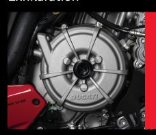
The 955 cc Superquadro twin of the Streetfighter V2 can achieve 153 hp at 10,750 rpm and maximum torque of 101.4 Nm at 9000 rpm.
